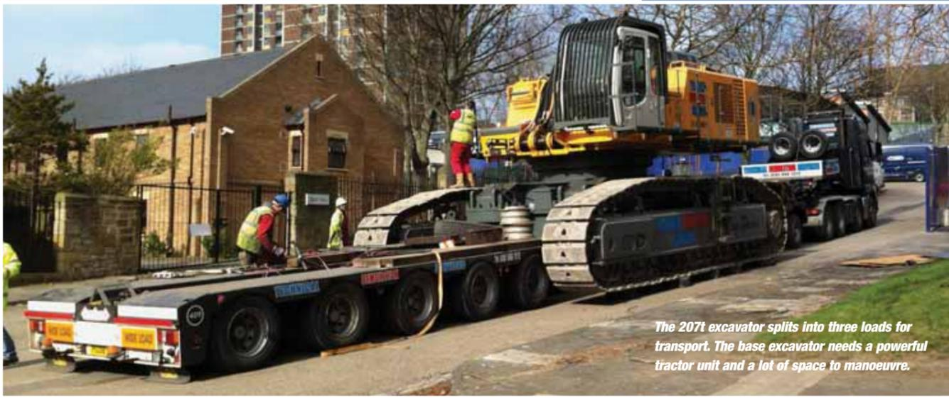
*The 207t excavator splits into three loads for transport. The base excavator needs a powerful tractor unit and a lot of space to manoeuvre.*
