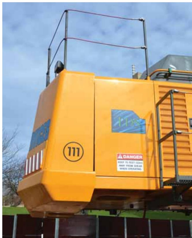
*The counterbalance is now hydraulically detachable. In front of it sits two internal 1000-litre water tanks for dust suppression.*
