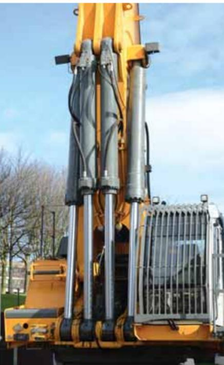
*Part of the conversion work included adding two extra main lift rams to provide the extra capacity to raise the 60t boom from the ground.*
