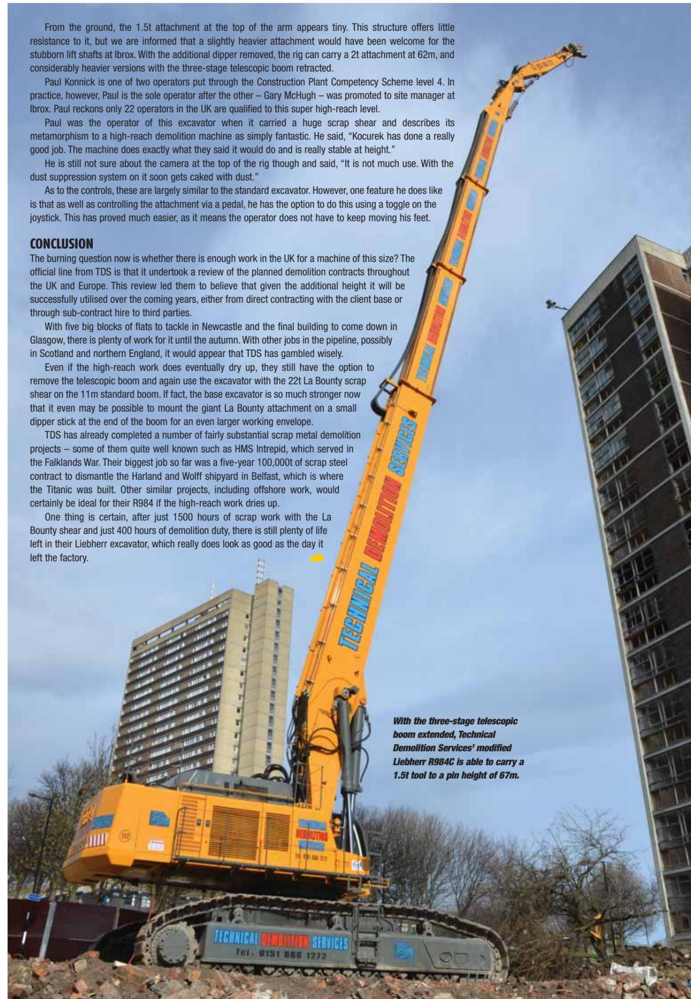
*With the three-stage telescopic boom extended, Technical Demolition Services' modified Liebherr R984C is able to carry a 1.5t tool to a pin height of 67m.*
